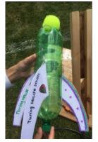
Our rocket had a simple yet thoughtful design. Increasing the mass at the front of the rocket (using a sand cone/tennis ball) means that the centre of mass is in front of, rather than behind, the centre of pressure, which allows the rocket to correct its alignment
